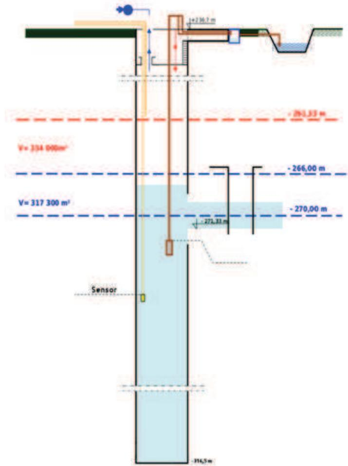
Figure 1. Typical flooded shaft with sensors
