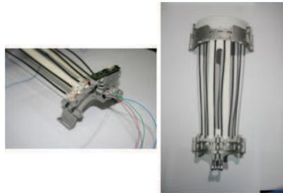
**Figure 5 - ALAS actuating device**
