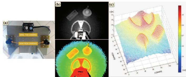
Fig. 7. (a) Set the cameras installed on the manipulator, mini-ToF and mini-RGB cameras. (b) Image of amplitude, and depth range of the mini-ToF. (c) Terrain surface mapping.
