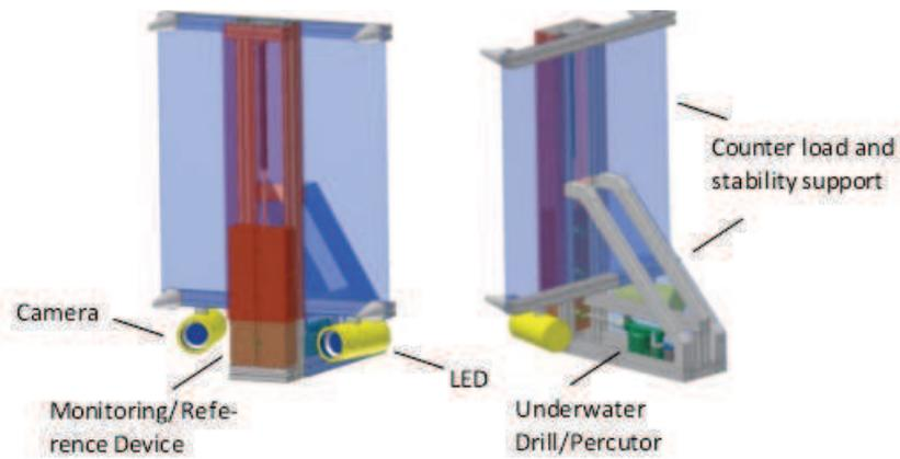
Fig. 3. Preliminary robotic system for sensors attachment
