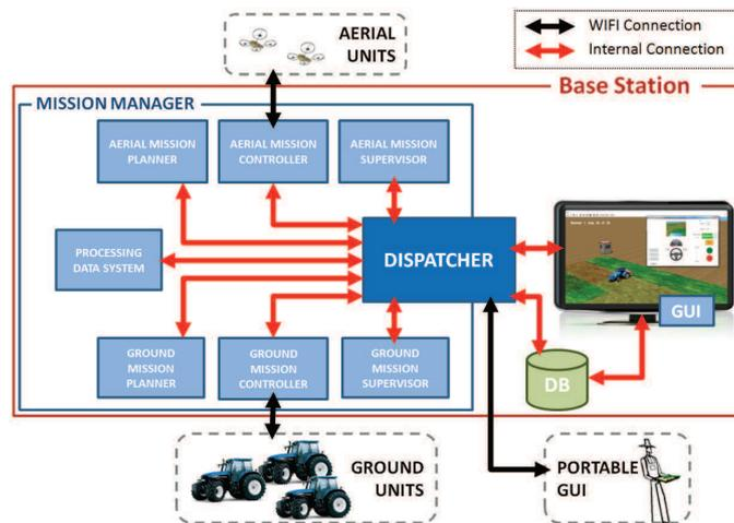
Figure 1. Internal structure of the Mission Manager as well as external systems with which it can interact.
