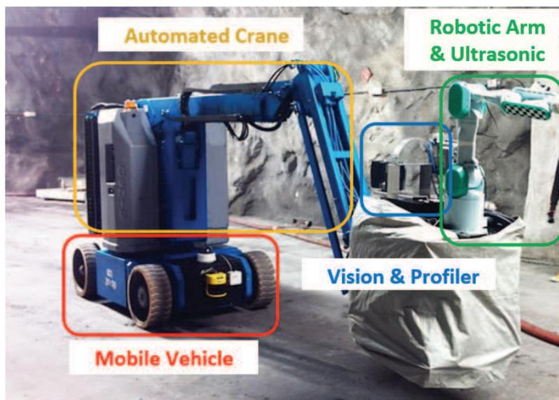
Fig. 2. ROBO-SPECT robotic system
