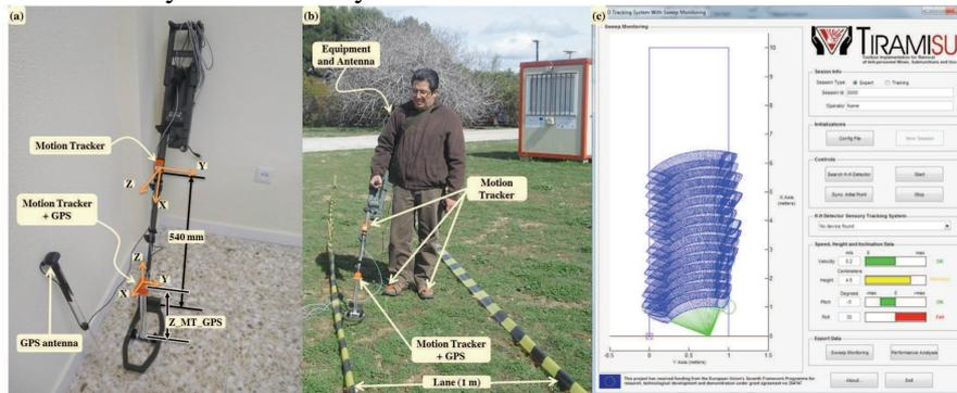
Fig. 1. (a) Compact metal detector with sensory system. (b) Apprentice with HHD training tool during an experimental test at CSIC premises. (c) GUI implemented in Matlab.
