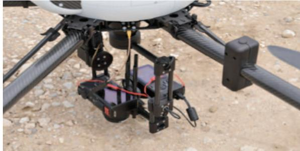
Fig. 2. Perception system on-board the drone
