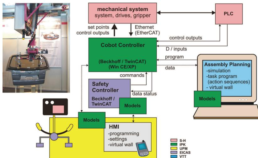
Fig. 4. Cobot control system architecture
