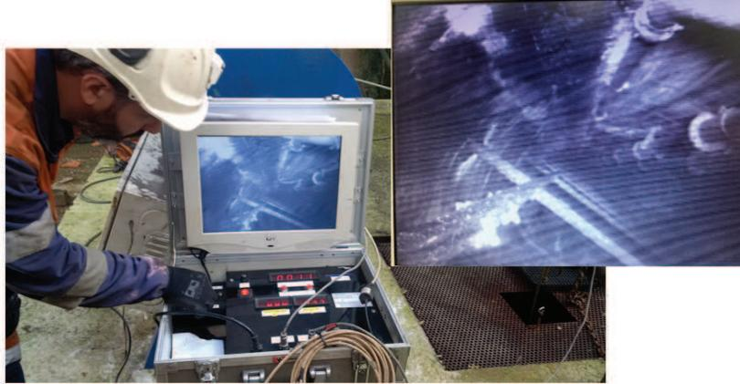
Figure 2. Ground monitoring system of the camera data in the Pozo Fondon (Asturias) flooded shaft
